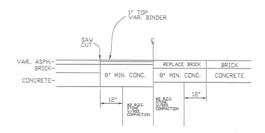
ASPHALT PAVEMENT W/BRICK & CONC. BASE
