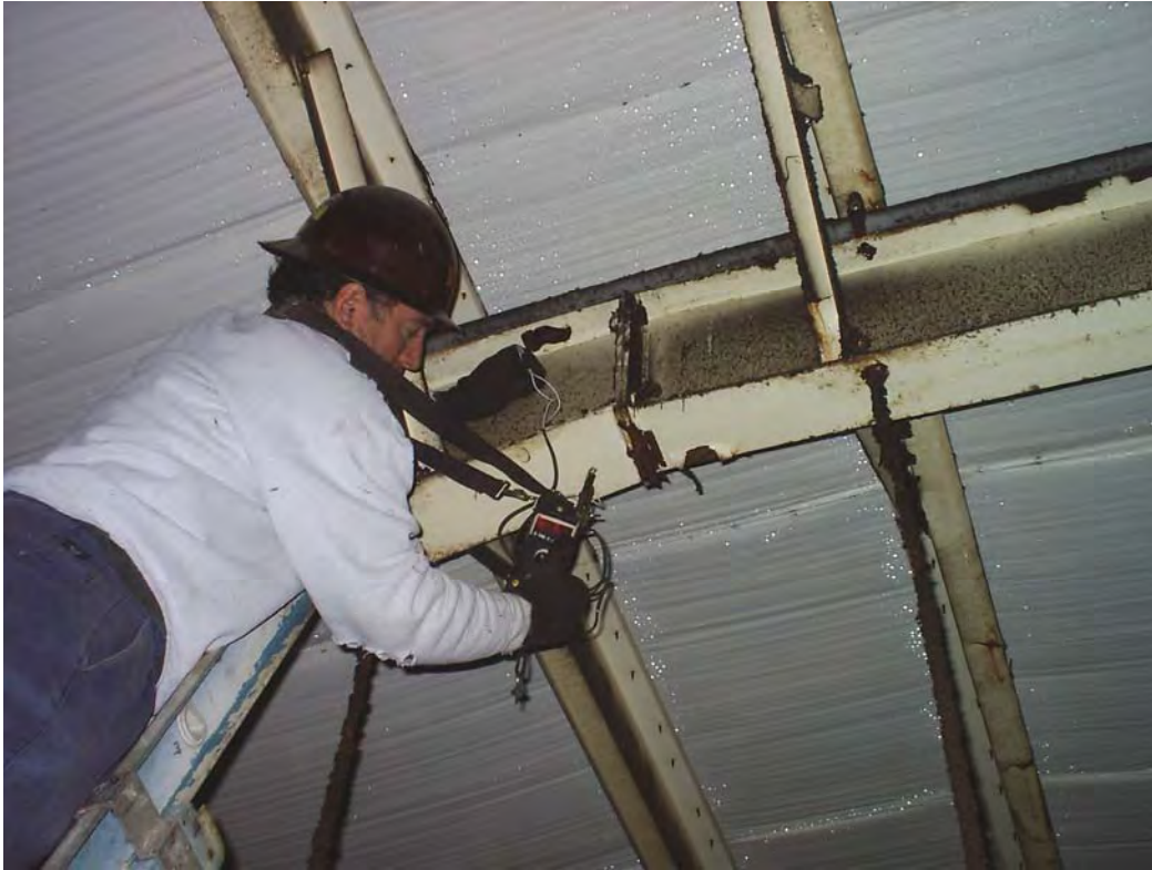
PHOTOGRAPH OF ULTRASONIC TESTING ACTIVITY, ROOF GIRDERS AND PURLINS, COMPOST AREA.
