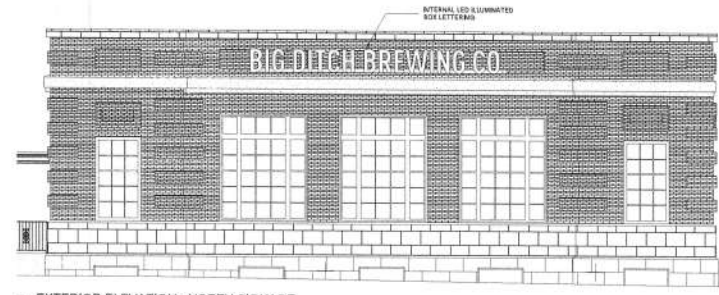
3 EXTERIOR ELEVATION - NORTH SIGNAGE 3/16" = 1'-0"
